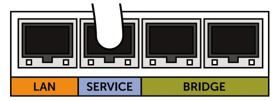
Connect the other end of the Ethernet cable to your workstation's Ethernet port.
